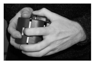
Extract the exhausted paper roll. You can use standard paper roll but you have to check before for its dimensions (max. 57mm ±1mm large and 48mm ±1mm roll diameter).
