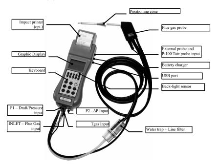
At the bottom of **EGA4** you can see all sampling probe connectors: gas inlet, pressure and draught input, thermocouple input for gas measurement and the 2<sup>nd</sup> pressure inlet connector.
