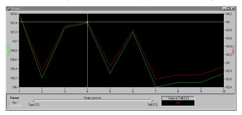
Activate the cursor and snap cursor to the desired parameter. Using the mouse you can move the cursor amongst the measurements.
